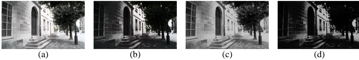
Figure 12. Subjective Performance Comparison for Quarter Power-consumed #2 Zahra Image: (a) HE Result, (b) CVC Result, (c) Difference between HE and Original, and (d) Difference between CVC and Original
