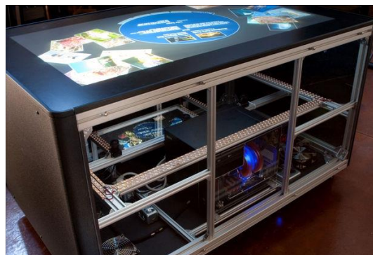
Figure 2. DIY MT-50 Multi-touch Table (Projector type)
