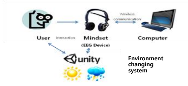
Figure 2. Process of EEG environment changing system.
