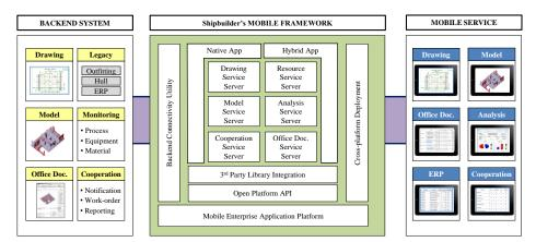
Figure 1. Shipbuilder's Mobile Framework
