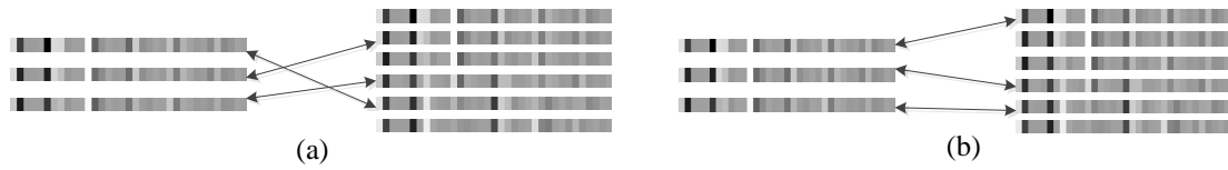
Figure 4. (a) Non-ordered and (b) ordered sequence matching methods
