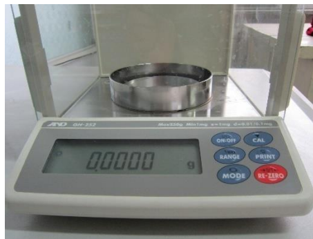
Figure 2. Photo of the Microanalytical Balance
