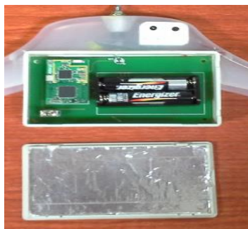
Figure 9. Manufactured Smart Hanger using the Electric Wave Absorber
