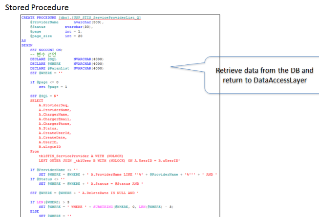
Figure 10. The database accessing procedure
