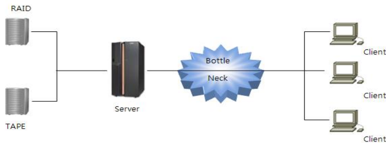
Figure 2. General storage server VS SAN structure
