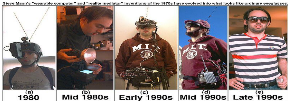
Figure 2. Evolution of Steve Mann's WearComp wearable computer from backpack based systems of the late 1970s and early 1980s to his current covert systems. [en.wikipedia.org]
