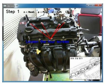
Figure 2. E-training AR System for Car Maintenance
