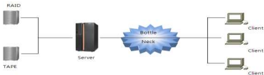
Figure 2. General Storage Server VS SAN Structure
