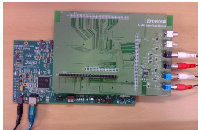
Figure 2. An implemented singing voice remover using DSP-TMS320C6713
