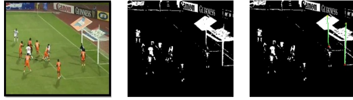
Figure 4. Hough transform for detecting the vertical goal posts
