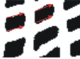
Fig. 2. The grid after application of the adaptive thresholding with marked sides of the segments.
