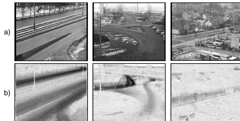
Figure 2. Determining usual movement paths; a) sample backgrounds from video recordings; b) images illustrating movement density in analyzed scenes (the darker pixel the higher density)
