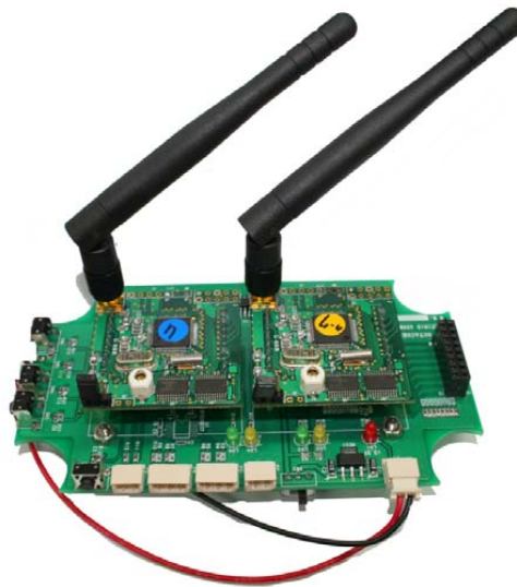
Figure 3. Developed interface board and RF board
