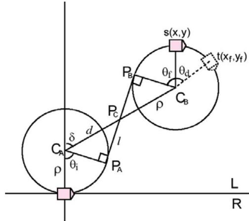
(Fig.5) The standard form of type LSR
