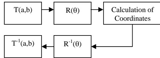
(Fig.2) Process of the coordinates transformation
