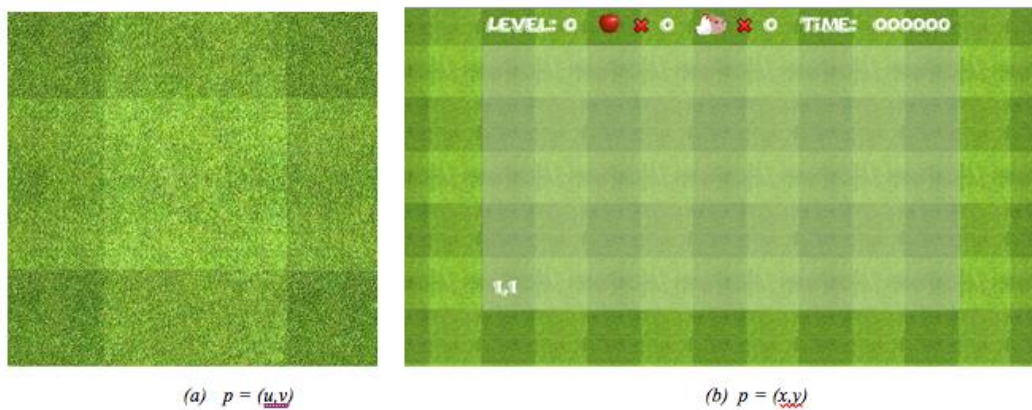
Figure 3. (a) 2D Image for the UV Wrapping. (b) Game Level after Uv Mapping is Applied and the Necessary Calculations Done
