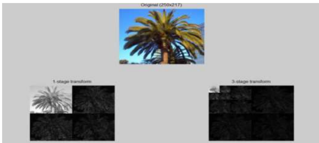
Figure 18. Wavelet Decomposition using Lifting based (Bi-orthogonal) DWT
