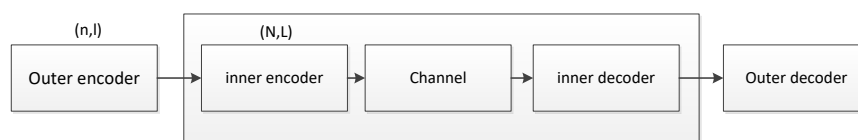
Figure 3. Schematic Diagram of Concatenated Coding
