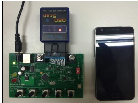
Figure 6. HW Configuration of Vehicle Simulation Using by OBD Scanner
