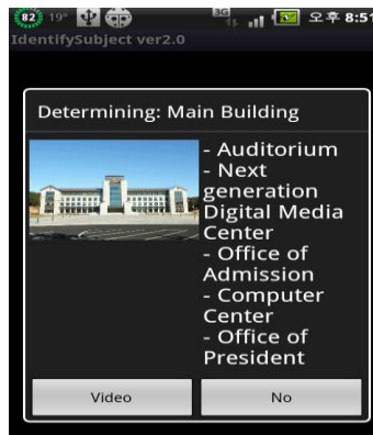
Figure 7. A Screenshot of the Campus Guide. It Detects Watching Status and Takes a Picture of the Building Automatically
