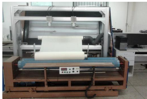
Figure 7. A Front View of the Architecture of a Typical Automated Textile Web Inspection System
