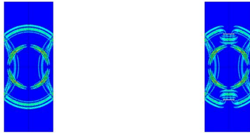
(a) Displacement Contour in the No Crack Plate (b) Displacement Contour in the Crack Plate
