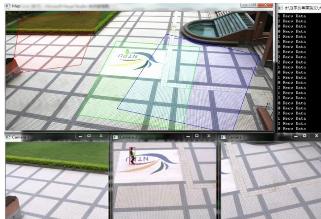
Figure 6. Object Tracking with Mixed Configuration of Overlapping and Non-Overlapping FOV Scenario: Object #8 Passes through the Blind Region between Camera 1 and Camera 2
