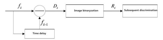
Figure 2. The Schematic Diagram of the Frame Subtraction Method
