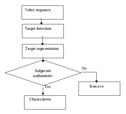
Figure 1. The Block Diagram of Target Detecting and Picking-Up
