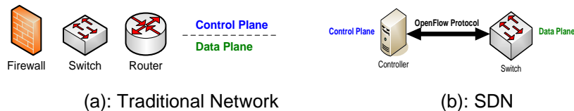
Figure 1.1. Control Plane & Data Plane in Traditional Network vs SDN
