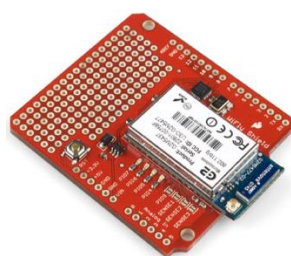
Figure 7. The WiFly Shield Equips our Arduino the Ability to Connect to 802.11b/g Wireless Networks
