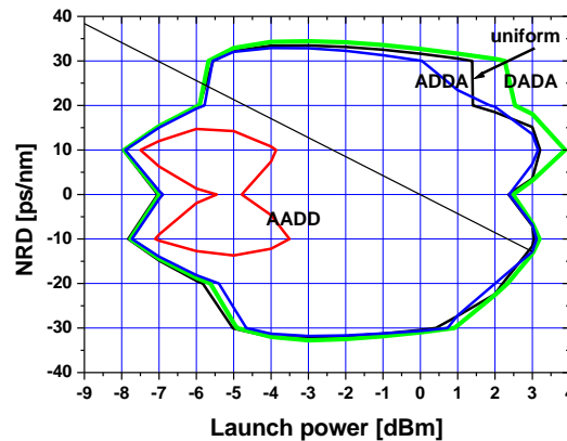
Figure 4. The Effective NRD Ranges of the Worst Channel Transmitted in 50 Fiber Spans as a Function of the Launch Power
