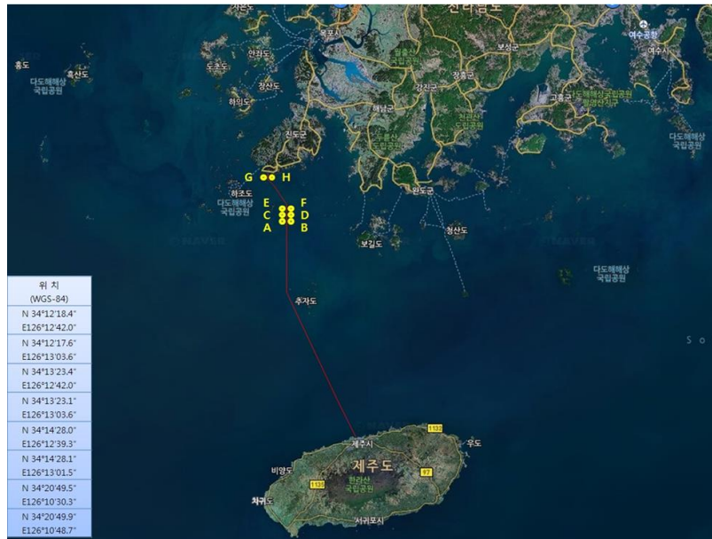
Figure 19. Positions of the Light Buoys Along the Jindo - Jeju Undersea Power Cable
