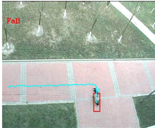
Figure 8. The Shape Aspect Ratio Changed when a Person Fell Downward
