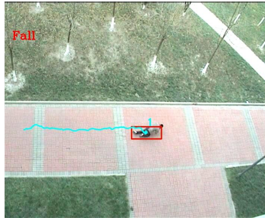
Figure 6. The Shape Aspect Ratio Changed when a Person Fell Forward
