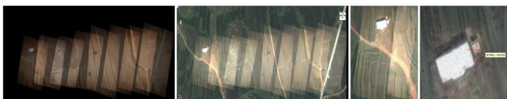
(a) Results of the Joints of the Aerial Photos (b) Results of the Matching of the Aerial Photos and the Digital Map (c) Details of the Matching (d) Obtain the Coordinate Information
