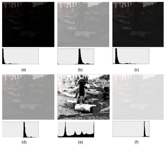
Figure 5. Results Comparison of Different Methods Operated on "Beach" Image. (a) Original Low Illumination Image, (b) The Enhanced Result Using our Method, (c) The Enhanced Result Using Method in [4]. (d) The Enhanced Result Using Method in [8], (e) The Enhanced Result Using HE, (f) The Enhanced Result Using Method in [6]
