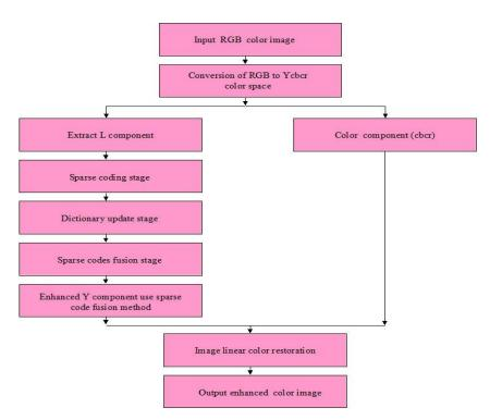
Figure 1. A Block Diagram of the Proposed Sparse Code Fusion Method
