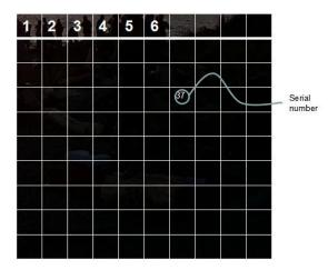
Figure 3. The Images of Training Data-Set are Divided into Patches which have their Own Serial Number to Record the Coordinate Position
