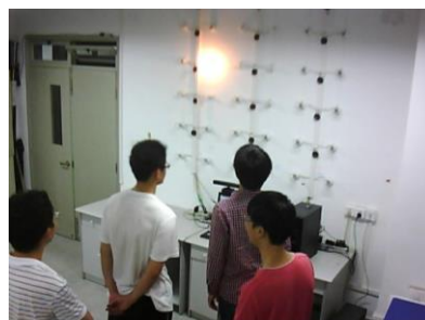
Figure 2. An Example of Face Orientation Estimation Based HCI: A Lamp on the Wall is Turned on According to the Face Orientation of One User
