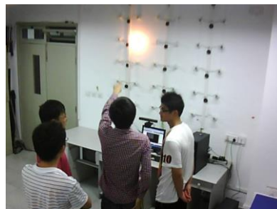
Figure 4. An Example of Hand Pointing Based HCI: A Lamp on the Wall is Turn on According to the Hand Pointing
