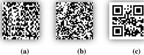
Figure 7. The Resultant Images of the First Stage, (a) Master Share, (b) Secret Share, (c) Reconstructed QR-Code Watermark
