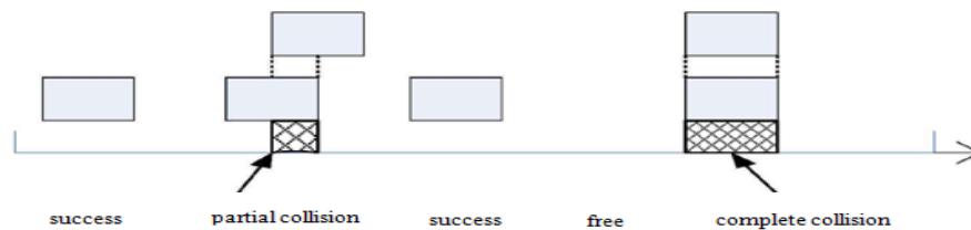
Figure 2. Pure ALOHA Algorithm in Information Time Division Multiple Access Diagram
