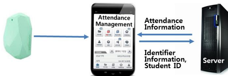
Figure 3. Operation of BLE Beacon
