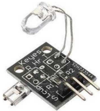
Figure 2. Infrared transmitter and received sensor pair clipped to the finger
