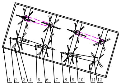
1,3. Frame 2,5,8. Cleaning element I 4. Deliver roller 6. Second order leaf- stripping roller 7. Bearing chock 9. First order leaf-stripping roller 10. Transmission chain 11. Cleaning element II 12. Inlet roller
