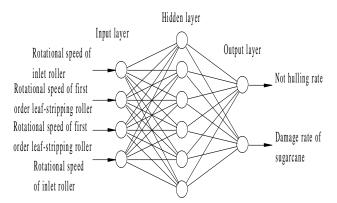
Figure 3. The Prediction Model of Leaf-Stripping Device
