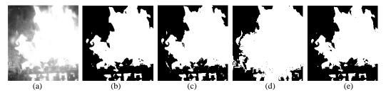
Figure 4. Segmentation Results of Mine Fire Disaster Image. (A) The Mine Fire Disaster Image (B) Roberts (C) Sobel (D) Log (E) Our Method
