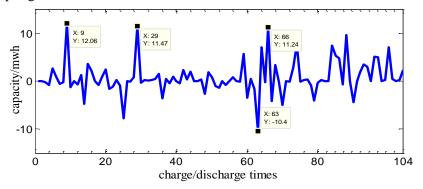
Figure 11. Charge and Discharge Capacity Curve of Storage System
