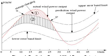
Figure 1. Prediction Error of Wind Power Output
