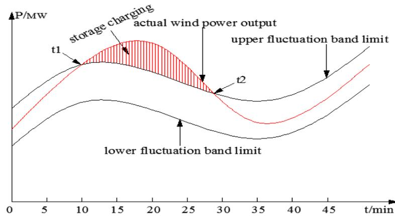
Figure 2. Fluctuations of Wind Power Output
