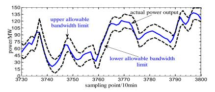
Figure 9. The Correlation between Wind-Storage Power Output and Allowed Bandwidth with Storage Capacity
