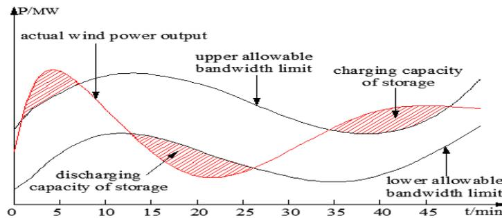
Figure 5. Caculation of Optimal Storage Capacity
