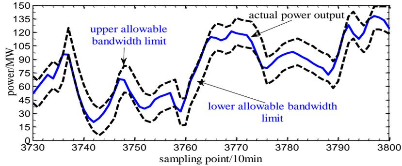
**Figure 9. The Correlation between Wind-Storage Power Output and Allowed Bandwidth with Storage Capacity**
