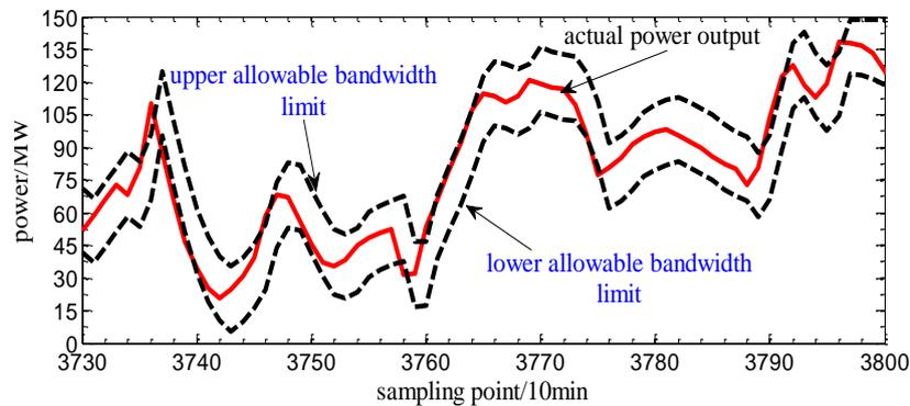
Figure 8. The Correlation between the Actual Power Output and Allowed Bandwidth with No Storage Capacity
