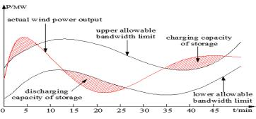
Figure 5. Caculation of Optimal Storage Capacity
