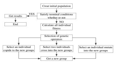
Figure 4. The Basic Flow Chart of Genetic Algorithm
