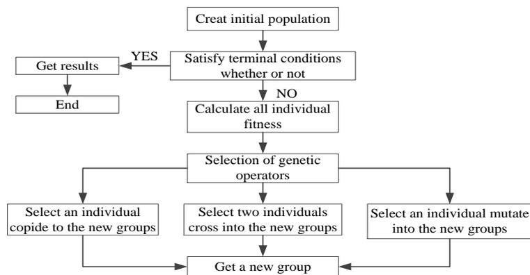
Figure 4. The Basic Flow Chart of Genetic Algorithm
