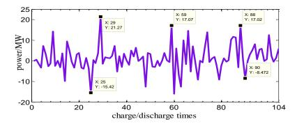
Figure 10. Charge and Discharge Power Curve of Storage System
