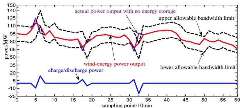
**Figure 12. Wind-Storage Power Output and Charging Curves with Optimal Storage Capacity**
