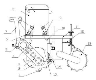
Rotary tillage mechanism 2. Bottom plate 3. Side gear box 4. Fertilizing tube 5.
