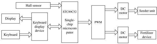
Figure 4. General Device Block Diagram
