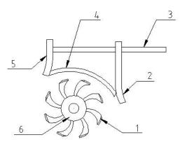
1. Rotary blade 2. Seeding tube 3. Rack 4. Breast board 5. Fertilizer feeding tube 6. Tool apron
