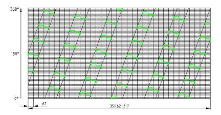
Figure 3. Expanded View of Blade Arrangement
