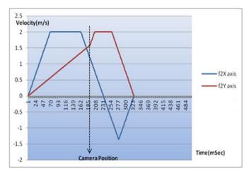
Figure 6. Velocity Graph of the Fly2-Motion
