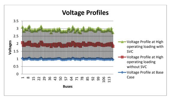
Figure 8. Voltage Profiles for 118 Test Bus Systems by GSA
