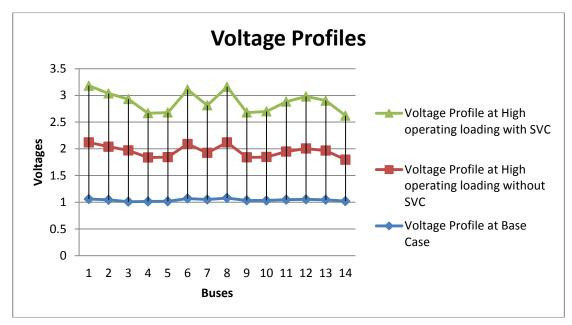
Figure 4. Voltage Profiles for 14 Test Bus Systems by GSA
