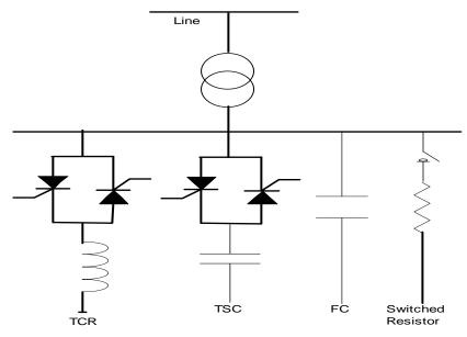
Figure 1. Basic Structure of A SVC
