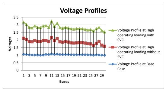
Figure 6. Voltage Profiles for 30 Test Bus Systems by GSA
