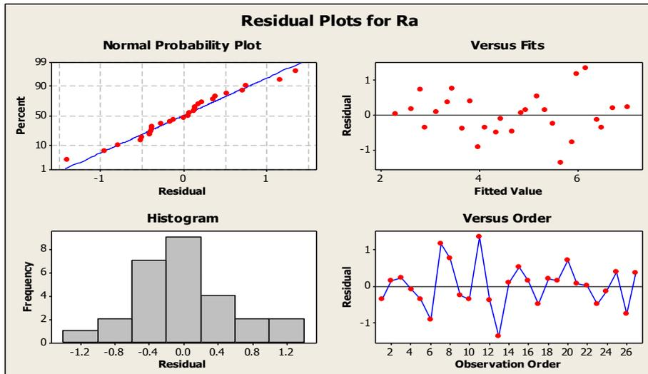
Figure 3. Residual Plots for  $R_a$
