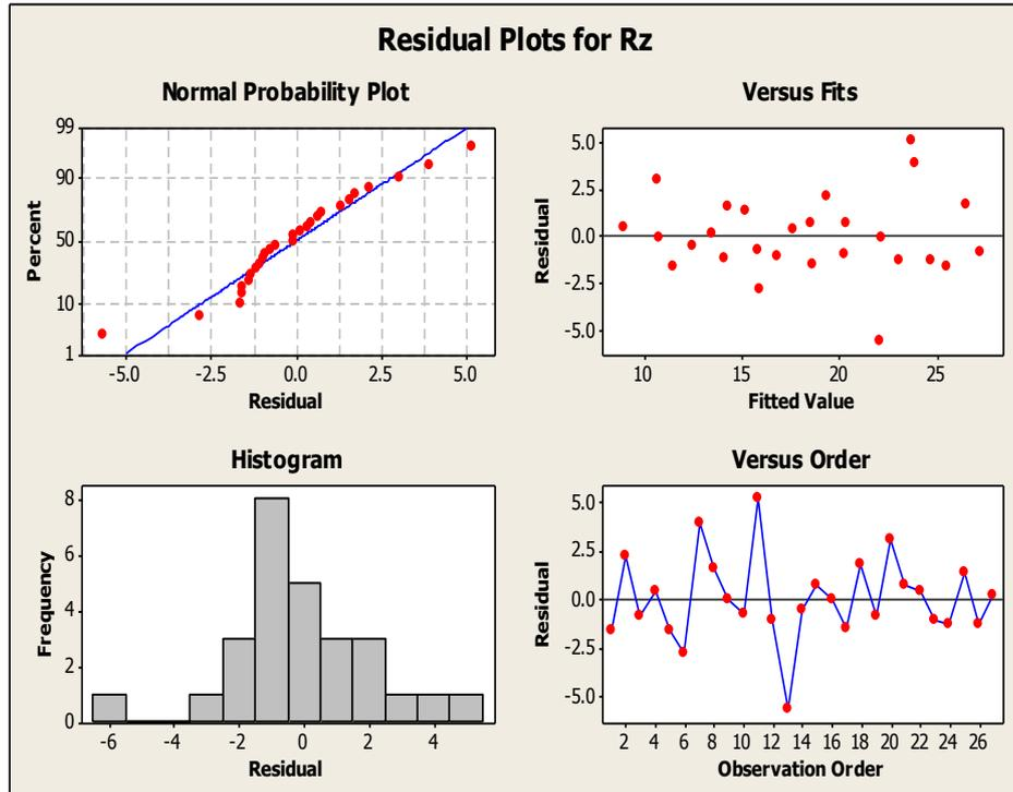
Figure 5. Residual Plots for  $R_z$
