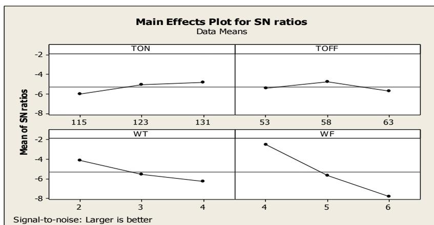
**Figure 2. Main Effect Plot for S/N Ratios of GRG**
