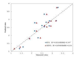
Figure 2. Comparison between Predicted and Measured Values of Two Retrieving Models Based On the TM Sensor
