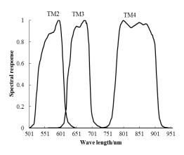
Figure 1. Landsat TM-5 Satellite Sensors TM2, TM3, TM4 Spectral Response Functions
