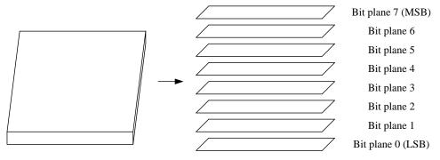
Figure 1. Bit Plane Slicing Representation of an Image (N=8)
