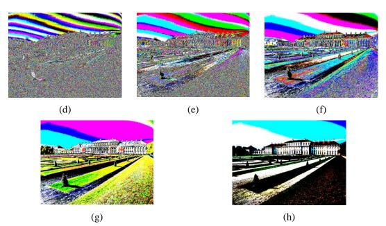
Figure 3. Separate Plane Example of Bit Plane Slicing on 8-Bit Color Image: 31st LC Image: (A) Bit Plane 1 (LSB), (B) Bit Plane 1, (C) Bit Plane 2, (D) Bit Plane 3, (E) Bit Plane 4, (F) Bit Plane 5, (G) Bit Plane 6, And (H) Bit Plane 7 (MSB)
