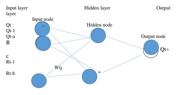
Figure 14. A Three Layer MLP Neural Network Method
