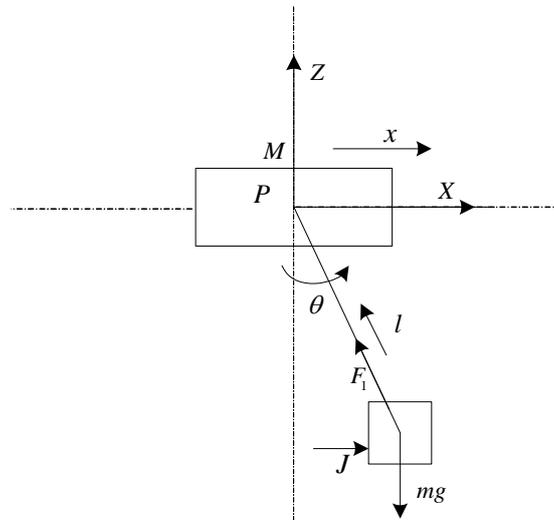
**Figure 2. The Plane Diagram Of Suspended Servo System**
