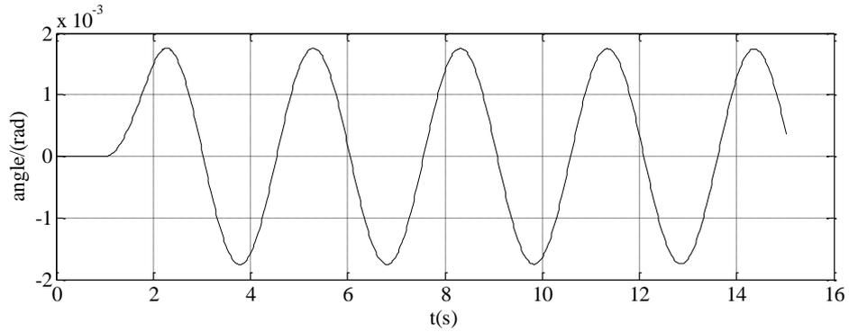
**Figure 6. The Curve of Swing Angle Without Controller**
