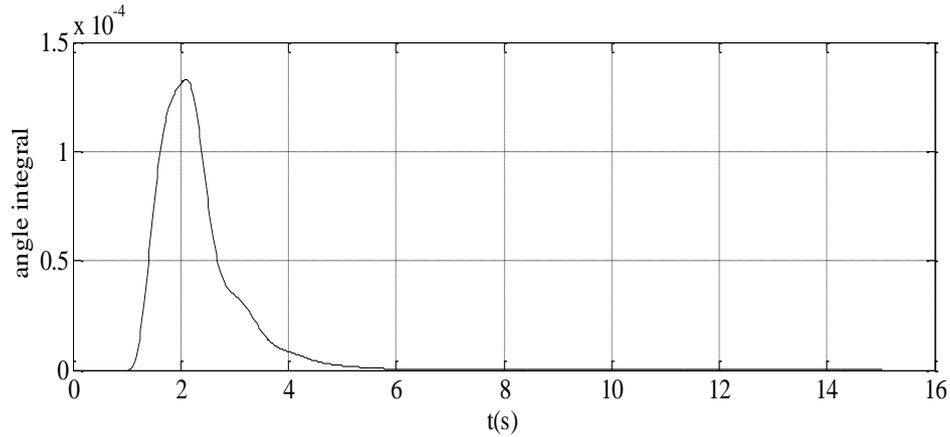
**Figure 9 The Curve of Sling Swing-Angle Integral With Servo Control**
