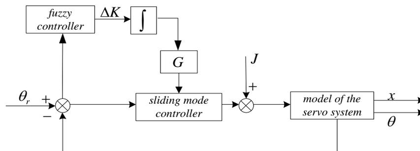
**Figure 3. The Structure of the Control System**
